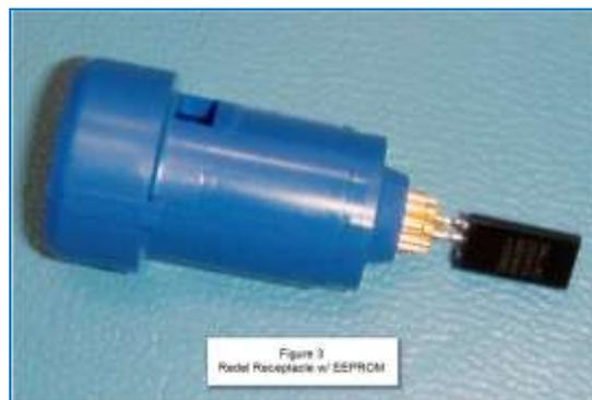
**Integrated Electronics:** The medical device designer may also consider custom circuits for noise filtering or EMI (Electromagnetic Interference) suppression, signal conditioning, temperature sensing, or circuit protection integrated on a PCB within the connector. In this way the electronics will be in close proximity to the probe or sensor, or noise source improving system performance.
