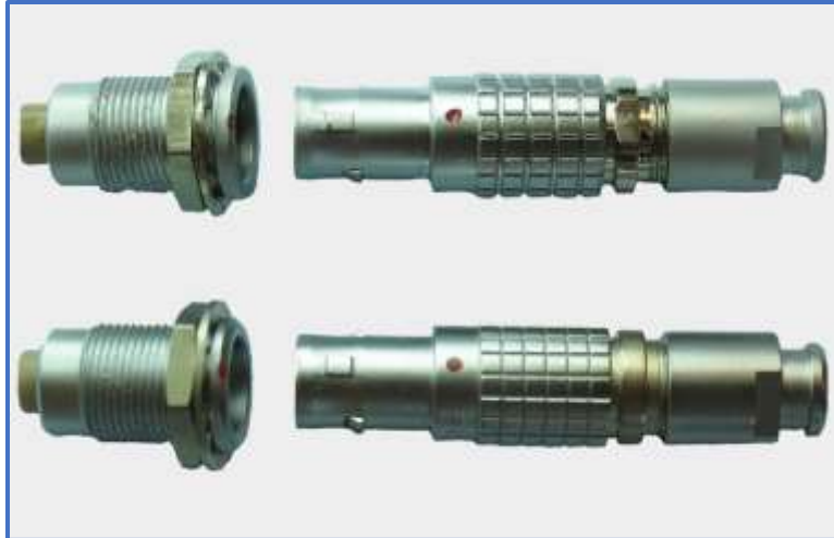
FIGURE 2: LEMO B SERIES: IMAGE ON TOP IS COUNTERFEIT AND BOTTOM IS AUTHENTIC LEMO B SERIES: NOTE ON COUNTERFEIT CONNECTOR THE RED DOT IS OUT OF ALIGNMENT AND THE FINISH IS INFERIOR.
