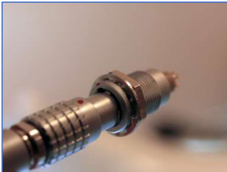
FIGURE 3: COUNTERFEIT CONNECTOR: THE RECEPTACLE AND THE PLUG CAN MIS-MATE, POTENTIALLY CAUSING MECHANICAL DAMAGE TO THE CONTACTS AS WELL AS POSSIBLE DAMAGE TO THE SIGNAL AND POWER WITHIN THE EQUIPMENT
