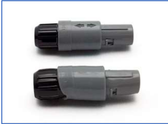
FIGURE 1: TOP: AUTHENTIC REDEL. BOTTOM: COUNTERFEIT. COUNTERFEIT REDEL - 150°C MAX OPERATING RATED TEMPERATURE. CLEARLY THESE MATERIALS ARE SUB-STANDARD
