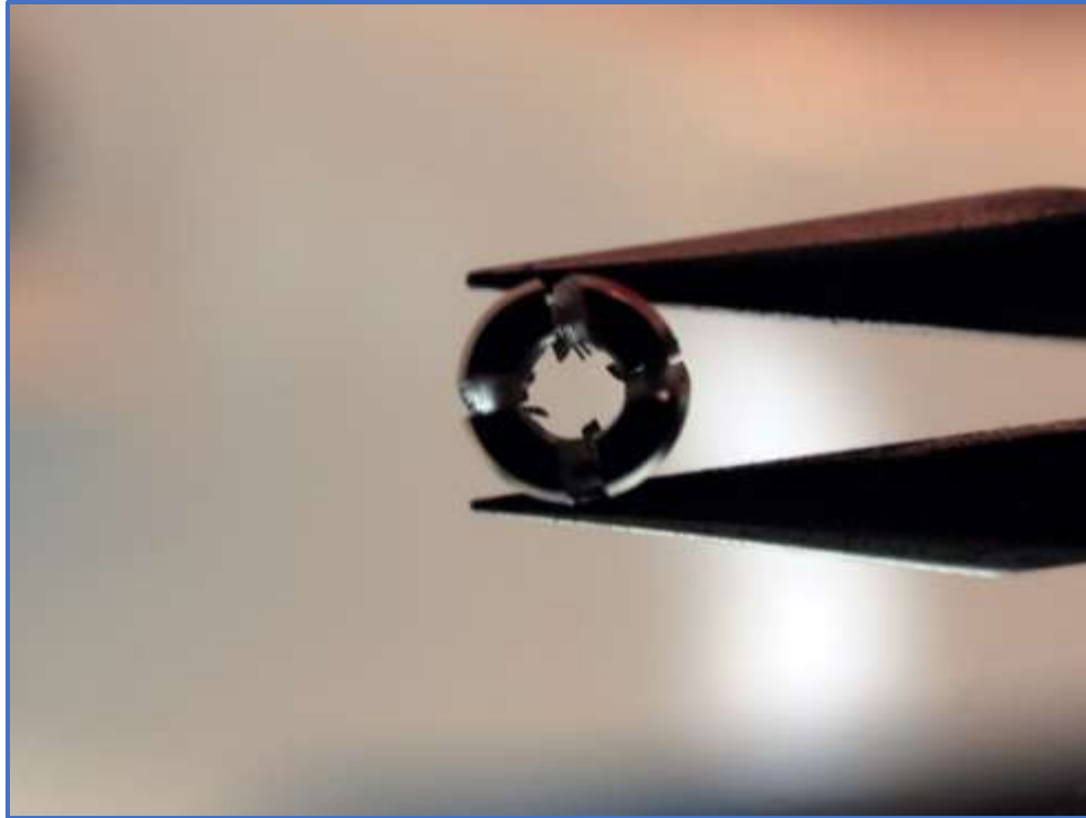
FIGURE 4: COUNTERFEIT CONNECTOR: THIS IS AN INTERNAL METAL COMPONENT (COLLET) THAT STILL HAS BURRS LEFTOVER FROM THE MACHINING PROCESS. IF ONE THESE BURRS FLAKED OFF IT COULD GET INTO THE ELECTRICAL CONTACT AREA AND POTENTIALLY CAUSE A SHORT.
