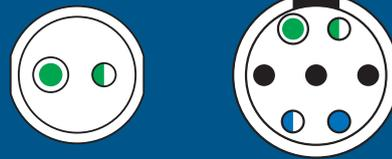
**Note:** <sup>1)</sup> AWG 26, please check wire construction wire section should be less than 0.14 mm<sup>2</sup>
